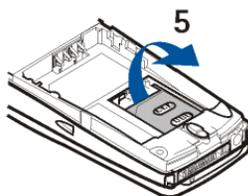
4. Insert the SIM card into the SIM card holder (6). Make sure that the SIM card is properly inserted and that the golden contact area on the card is facing downwards.
